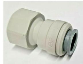
You can use 15mm push fit plumbing but you may need to modify the fitting so the washer seals against the flat face of the tank. Alternatively you can get 12mm fittings for the tank with a 12mm-15mm reducer.
