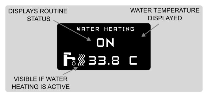
As with air heating, activate with the 'on' button and stop with the 'off' button. When the desired water temperature has been achieved the heater will be shut down and the routine ends.
