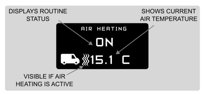
If the temperature goes over the set point by 2 degrees and the heater is on its lowest setting, the heater will be turned off. However, the routine will stay on and when the temperature drops to 3 degrees below the set point, the heater will be turned on again.
