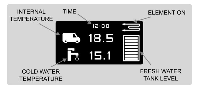
The fresh water tank level is only displayed if the sensor is connected.
