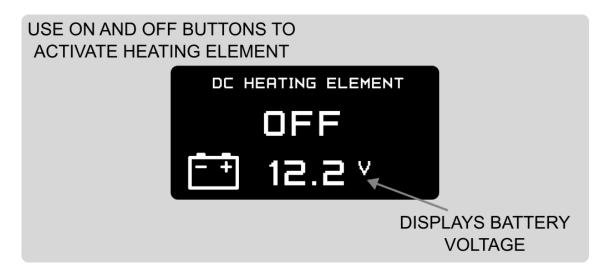
You can change the voltages at which the element is turned on and off. To modify the voltages:
