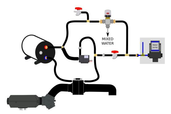
There is an extra drain valve at the hot inlet to the thermostatic mixer. This ordinarily remained closed, but if you wish to drain the main tank, then you open this valve. This allows air back into the tank when draining the tank, else there will be an airlock and the tank won't drain properly.
