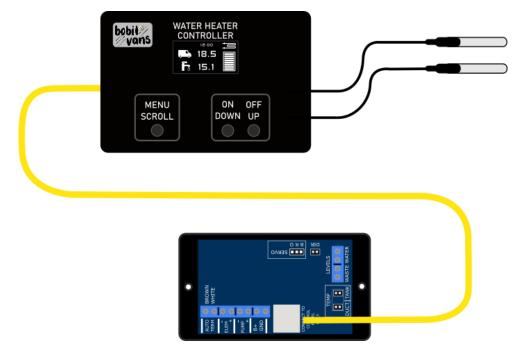
The two sensors from the master controller are for measuring the internal and external temperatures. The internal sensor should be mounted high up in the main living space, away from any direct flow from the heater outlet duct. The external sensor can be mounted anywhere outside the vehicle but must be protected from moisture. We would suggest attaching it to the underside of the van with the provided rubber P-clip.
