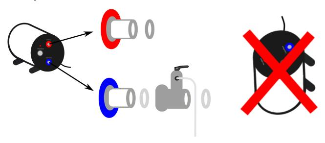
The tank cannot be mounted vertically.
