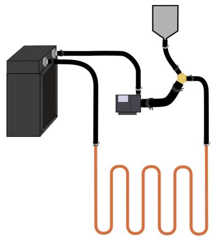
Fill the header tank with glycol and water in the appropriate mixture, following the instructions on the bottle.
