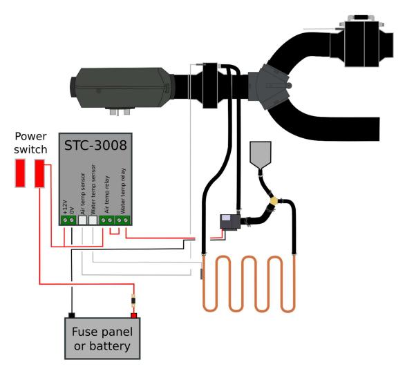
Set the temperature accordingly. Most domestic underfloor heating systems will run at 70 degrees. To set the air temperature turn on point to 40 degrees and the water temperature to 70 degrees, set the controller to the following values. Hold down the relevant arrow and when it starts flashing, adjust using the up and down keys.
