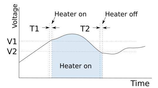
Note that for the element to stay on, you must have enough power coming in to maintain the voltage. If the element is turned on then immediately goes off, it is because the power supplies are not sufficient.
