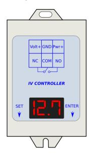
The controller will wait for the battery voltage to go above the programmed limit (V-1). When it does, it will wait for a short time delay (T-1) before switching on the relay. The relay will stay closed until the voltage drops lower than the second programmed limit (V-2), when it will start a second time delay (T-2) before switching the relay off.
